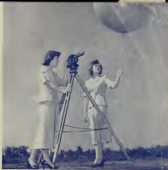
Pfc Ann Roach and Sgt Shirley Molisee work with theodolite and pilot balloon.
