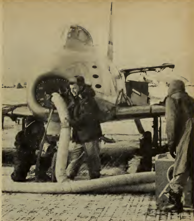
The freezing cold in Korea loses its bottle with ground crewmen, as they pipe 300-degree heat into an F-86 engine of the 4th Fighter Interceptor Wing in Korea. Using a portable heating unit and two hoses, the men melt ice on outside of the aircraft as well as heating the engine.
