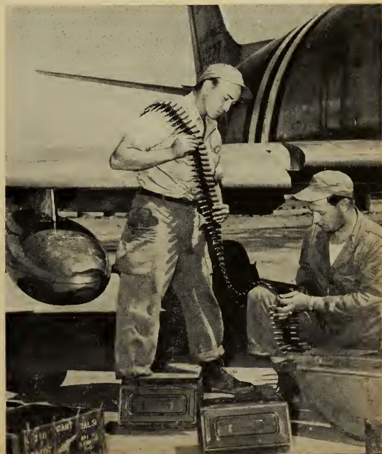
Armament technicians of the Fifth AF's 4th Fighter Interceptor Wing ready on F-86 for combat. S Sgt C. A. Norris (left) and T Sgt Joseph Adams, Jr., coil the belted caliber ammunition inside the containers which feed the guns. The ammunition will be used over "MIG Alley."
