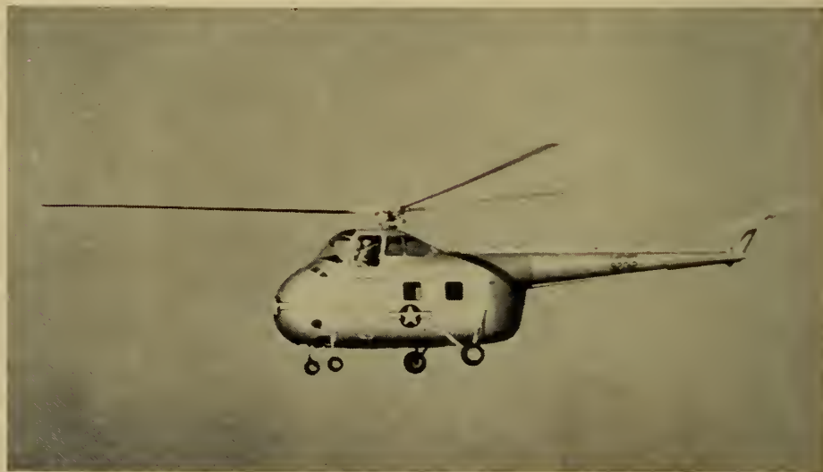
The Air Force's newest helicopter, the Sikorsky H-19, is designed as a search, rescue and liaison aircraft. It will transport eight litters and one attendant, or ten persons. The all-metal, three-bladed rotor atop the H-19 is driven by an R-1340 radial engine.
