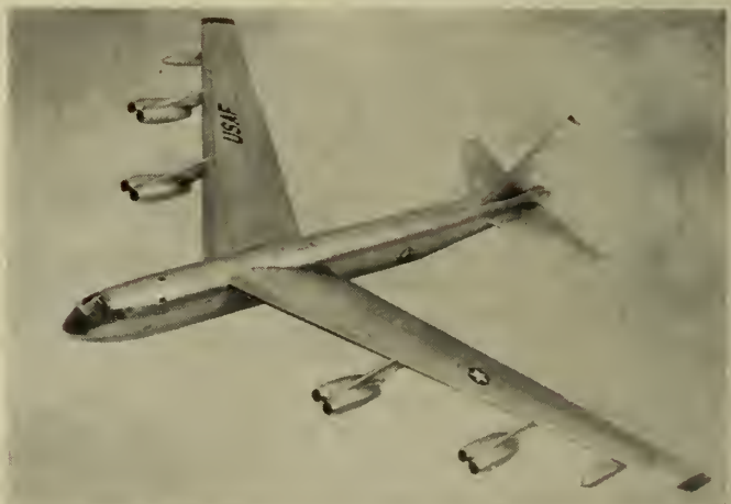
Model of new Boeing B-52 Stratofortress now in production at the Seattle plant of Boeing Airplane Company is shown above for the first time. Eight J-57 turbojet engines are mounted in four sharply raked-forward pods under the swept-back wing. Auxiliary fuel tanks are located under each wing tip.
