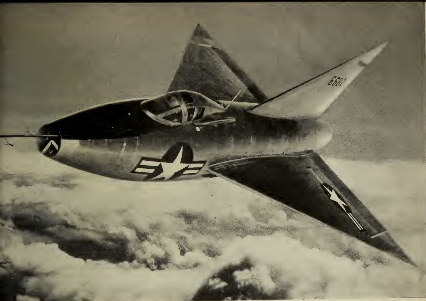
FIFTY YEARS AFTER MAN'S FIRST POWERED FLIGHT, THE AIR FORCE'S XF-92 WITH ITS DELTA WING DESIGN ILLUSTRATES THE PATTERN FOR THE FUTURE.
