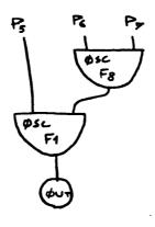
Note: here the rate at which the frequency controlling functions are scanned is determined by P7 (converted by P(7)=F/P(7)): it is divorced from the duration of the note; in effect these functions are scanned several times for one note length.
