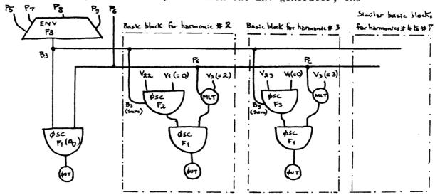
maximum amplitude of this component is determined by P5, and has to be smaller than 512. The output of the ENV generator is input-output block B3. B3 is used as amplitude input of the
