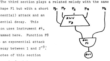
exponential attack time of 10 milliseconds which corresponds to a very sharp attack, and an exponential decay time varying between .5s and 2s. The tone quality reminds of a plucked string instrument.
